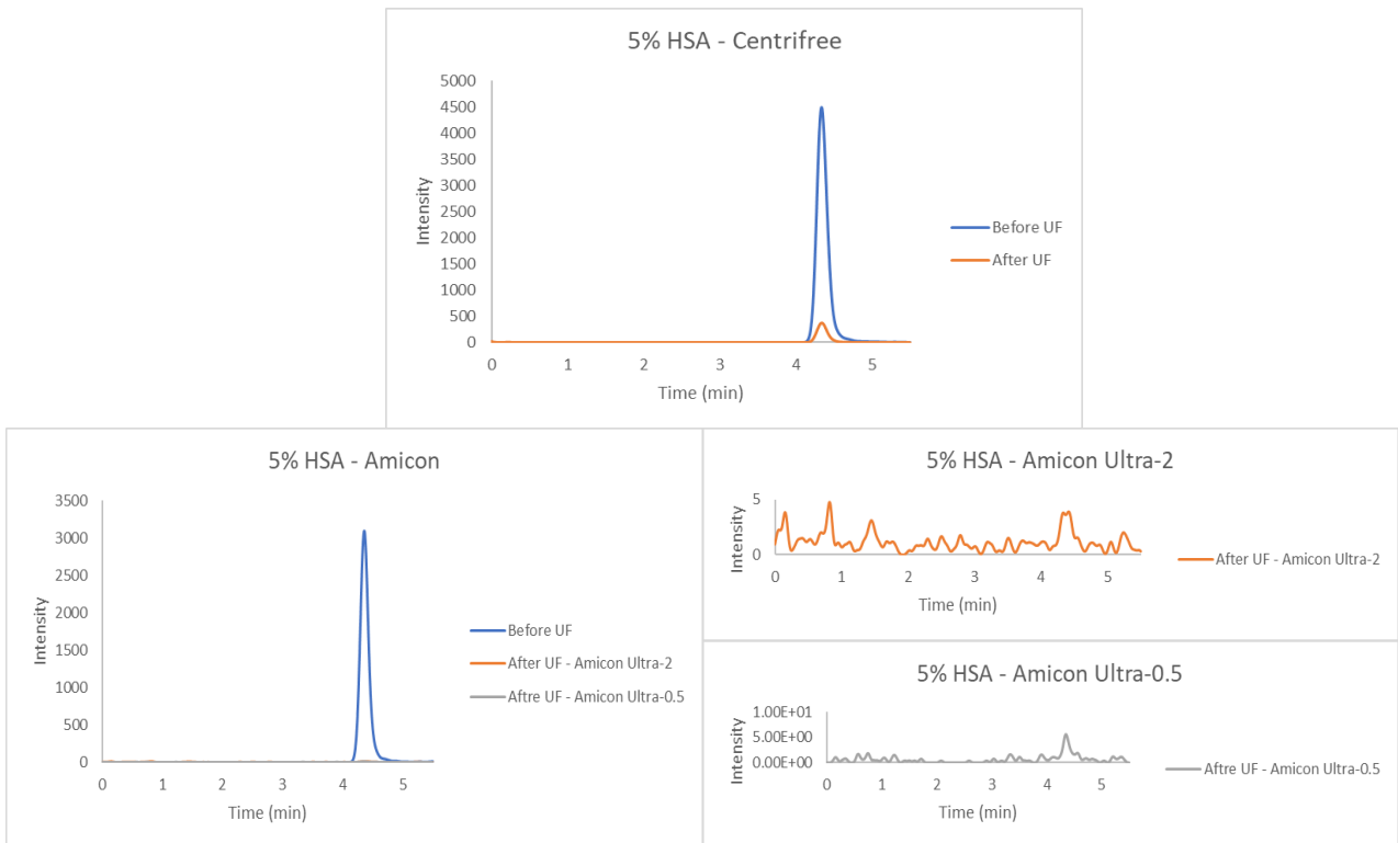
Fig. 2. Representative chromatograms of a 125 ng/mL CVD sample in 5% HSA before and after ultrafiltration (UF) using Centrifree vs. Amicon Ultra devices
